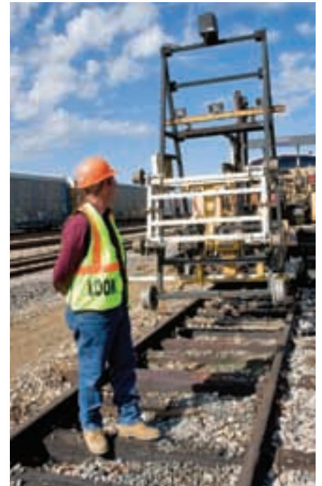
Pete standing in front of a “track tamper,” one of the machines he uses on the tracks.
