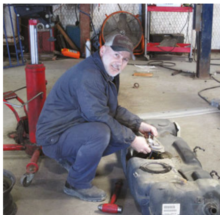
Eric Trojacek, owner of Eric's Garage, works on replacing a fuel pump.
